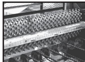
A close up of the iron rollers on the convoluting machine that's used to produce SonoMatt acoustic foam.
