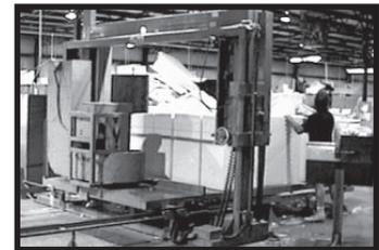
The slitting machine cutting a bun down into smaller blocks that'll then be cut into finished Auralex products.
