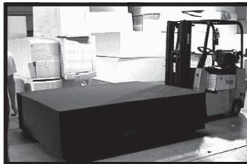
This is a bun that's been blocked and is being moved over to the slitter.
