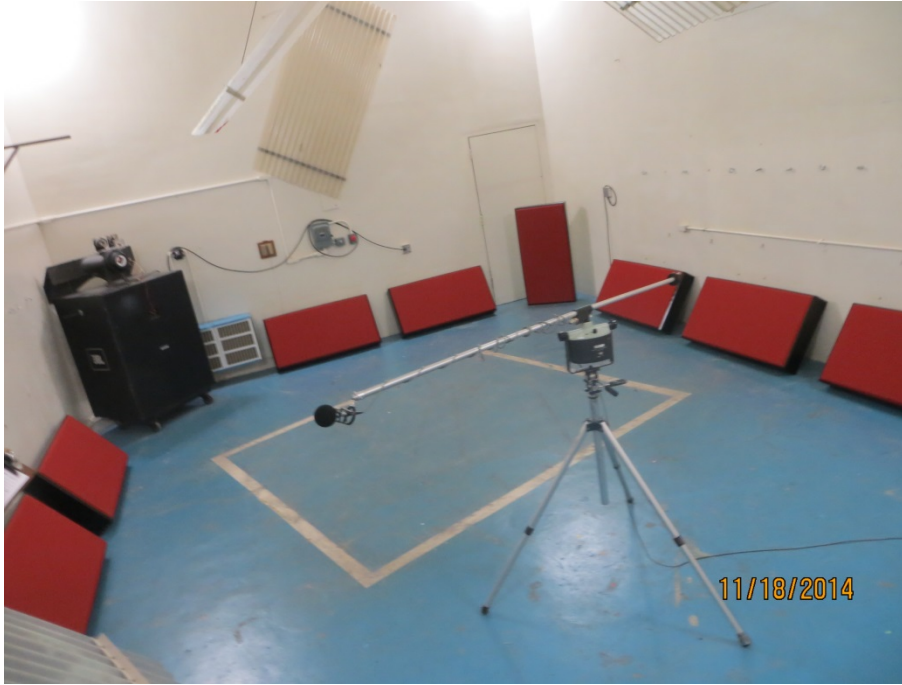
Figure 1 - Specimen mounted in the test chamber.
