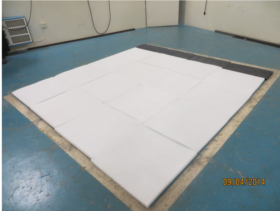
Figure 1 - Specimen mounted in the test chamber.
