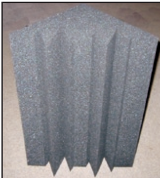
The LENRDs are 61 cm (24”) tall porous foam units that are stacked or glued into the room corners. The surface shape provides increased surface area at higher frequencies.
